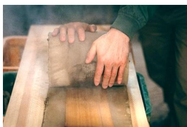
Winding the strip of wood onto the goro to bend
