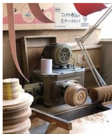
Wheel: Used to smooth the outside of round objects.
