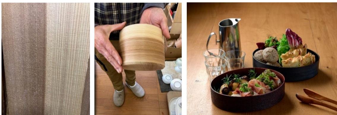
Heartwood and sapwood (The latter has newer growth rings.) Genpei brand utensil (mixture of sapwood and heartwood) Genpei
