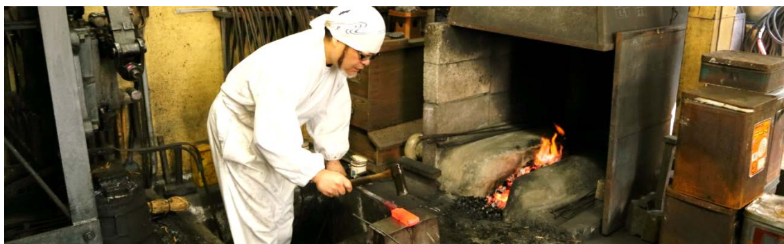
Kazuhiro Motegi, a pupil of Mr. Yamamura, forges a mixture of hard and soft steel.
