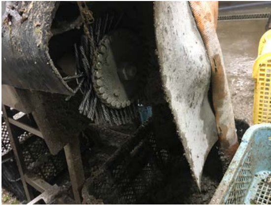
A special rotary brush to flick off barnacles
